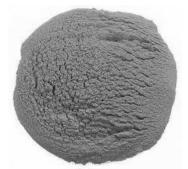
The chemical analysis of the coconut shell was done with Absorption Spectrometer (AAS)-Peckinhelma 2006 model. The particle size used was  $100 \ \mu m$ .
